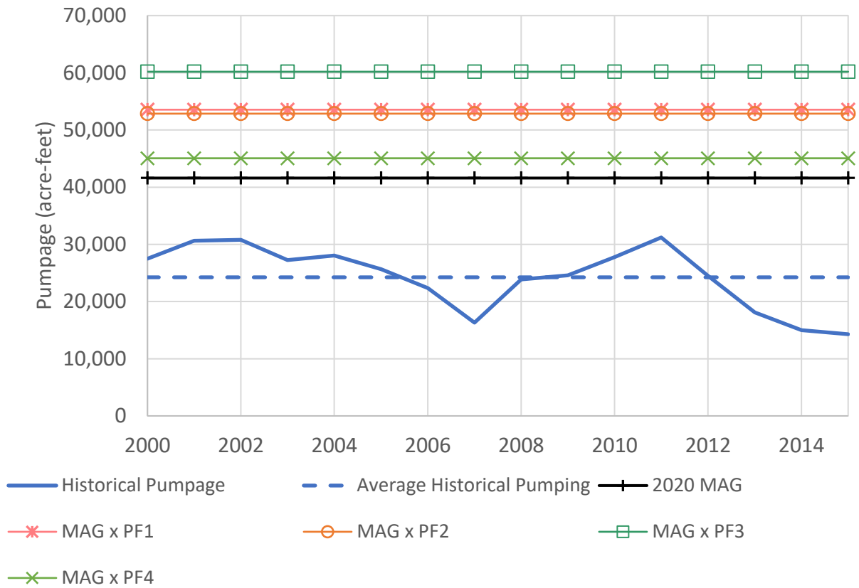
Figure 41. Historical Pumping, 2020 MAG, and 2020 MAG x Peak Factors for the Gulf Coast Aquifer in Waller County
